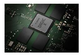
Dual processors have been a significant design feature of recent EOS-1D models, so the change to a single, new DIGIC X processor is a huge display of the confidence Canon engineers have in this unit's processing power.
