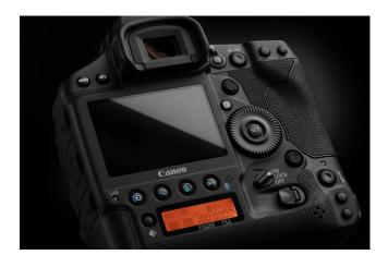
The AF-ON button now serves two roles — it's also the 1D X Mark III's innovative Smart Controller. Note that below the Smart Controller, the 8-way Multi-controller, seen on previous high-end EOS models, is also available. Both can be customized for quick manual movement of AF points or AF Areas.
