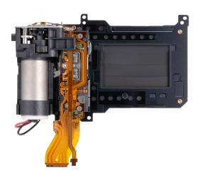
Simply stated, this is Canon's most durable and highest-performance mechanical shutter yet in a digital SLR. It's able to fire — in mechanical shutter mode — at up to 20 fps during Live View, and has been durability tested, along with the entire camera, to 500,000 exposures in tests by Canon engineers.
