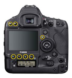
The EOS-1D X Mark III offers illumination of the buttons highlighted here in yellow (please note — the yellow highlighting in this graphic is strictly to show the buttons in question, and is NOT the actual illumination!).
